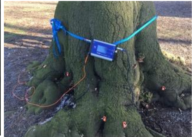
Mature Beech tree inspection with PICUS Tomograph, Abbey Park. Results show tree has advanced fungal decay
